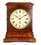
The Lantern and Longcase Clocks were powered by gravity, but around 1670 **Bracket or Mantle Clocks** appeared, and these were spring driven. This meant that they were more portable.
